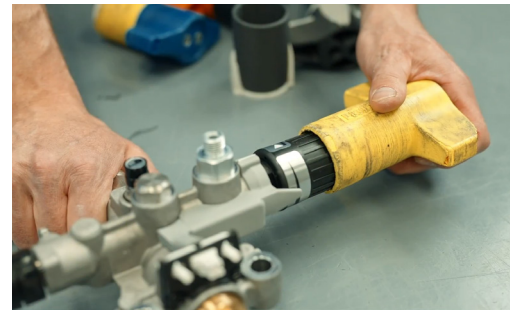
The old ABS hand tool (yellow) is shown, engaging the adjustment knob on a pressure control device.
