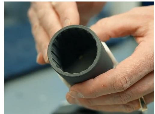
The 3D printed hand tool socket, showing the splines and the smooth as-printed surface finish.
